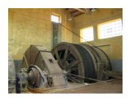
**The Winch Room** - the winding engine was used to move the cages up and down the shaft in order to transport the miners and the wagons.
