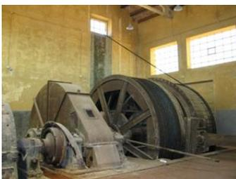
**Winding Engine House** - the winding engine was used to move the cages up and down the shaft in order to transport the miners and the wagons.
